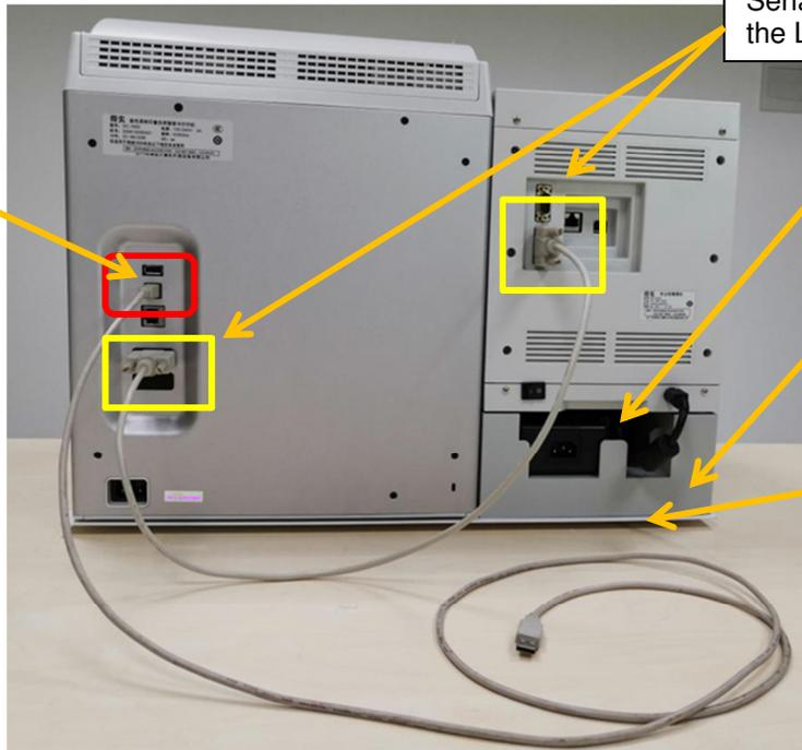
Serial Cable – Connection between the Laminator and the DC-7600 Printer
