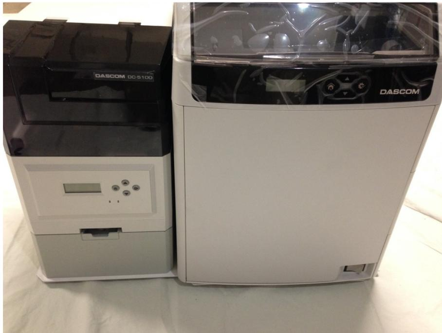
Gently lower the DC-5100 Laminator onto the stand, making sure to align it to the Stand.
