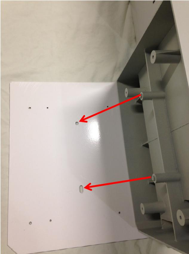
2) Place and align the Laminator Stand alignment posts, as noted, to the Mounting Plate.
