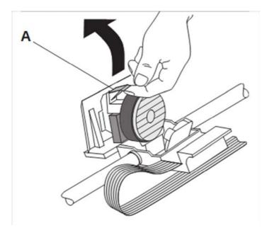
Raise the coloured insertion tongue **A**. Pull out and remove the coloured strip **A**.
