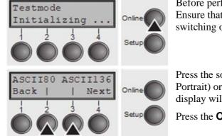
Before performing a self-test, your printer must be switched off. Ensure that paper is inserted. Keep the key **Online** pressed while switching on the printer, until **Testmode** appears on the display.
