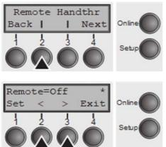
Use the < (2) or > (3) key to select the desired setting. Setting Options: **On/Off** Default Setting: **Off** Confirm the setting by pressing the **Set** key (1).
