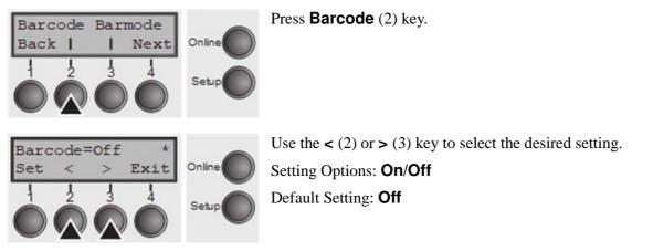
The definition and activation is performed by special sequences through the interface. Since this selection is possible for all emulations it must be noted that conflicts in sequence conformity with the selected emulation may occur. For this reason the barcode function can also be switched on and off by MTPL sequences. (The possible barcodes, LCP characters and the operation of these functions are described in the *Barcode Programmer's Application Manual*).
