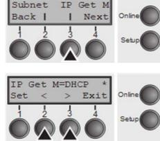
Use the < (2) or > (3) key to select the desired setting. Setting Options: **Static, DHCP, BOOTP** Default Setting: **Static**
