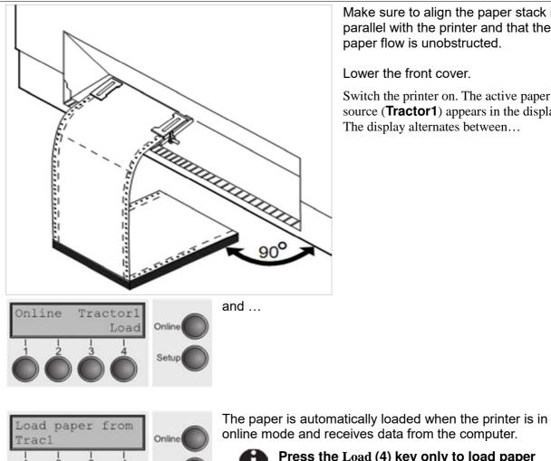
Make sure to align the paper stack in parallel with the printer and that the paper flow is unobstructed.
