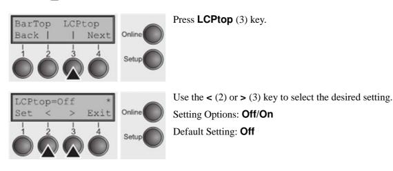
If this option is disabled (**Off**), then the printer advances paper 1/8 inch when exiting oversized characters. This characteristic is retained for compatibility with older products.
