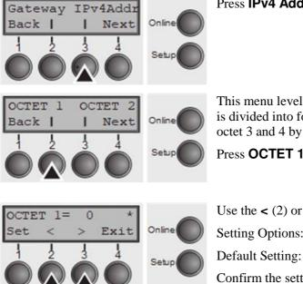
This menu level offers the possibility to set the IP address, which is divided into four digit groups (octet 1 to 4). You can activate octet 3 and 4 by pressing the **Next** (2) key.
