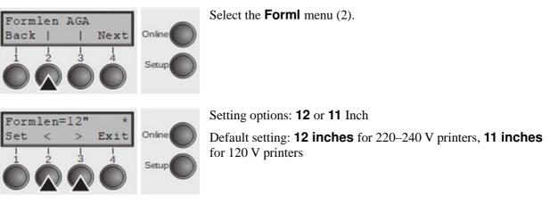
The value defined here is set in all five menus and for all paper paths. The setting made here is not changed by loading the default (factory) settings by pressing all four function keys.
