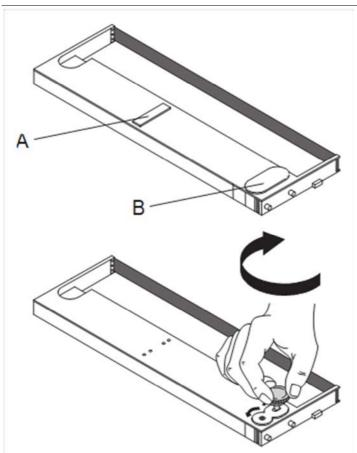
Slightly tilt the ribbon cassette forwards and thread in the ribbon between the coloured insertion tongue and the ribbon support (transparent plastic plate).
