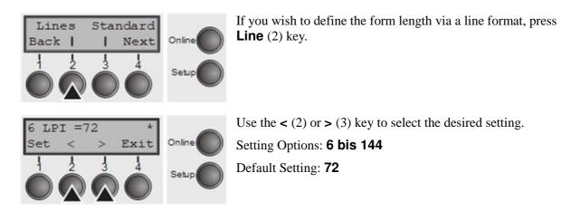
Sets the form length via line formats. Please note that the adjustment in **Lines** depends on the selected LPI. For example 8 LPI at a selected line number of 96 lines results in a formlength of 12 inches (96 lines/[8lines/inch]) = 12 inches). The selectable range is between 3 and 21 inches, i.e. for 2 LPI from 6 to 42 lines and for 12 LPI from 24 to 262 lines.
