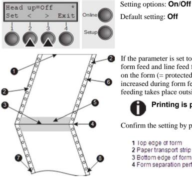
If the parameter is set to **On**, the printhead gap increases during form feed and line feed four lines before and after the perforation on the form (= protected zone). The printhead gap is always increased during form feeding past the perforation even when feeding takes place outside the protected zone.
