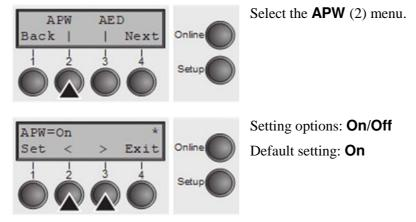
If **APW=On**, the printer is in the standard mode and truncates all data located beyond the right-hand and left-hand paper edge. These print data are lost.
