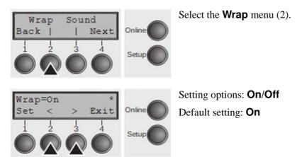
**Wrap = On**: If more characters than can be printed are transmitted per line, the characters which cannot be printed on this line are printed at the beginning of next line.
