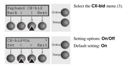
**CX-bid = ON** sets the parallel interface of the printer to bidirectional mode (IEEE 1284, Nibble mode), e.g. for Windows Plug & Play.
