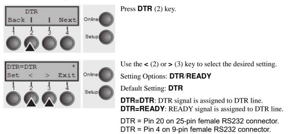
Confirm the setting by pressing the **Set** key (1). Press the **Next** key (4) to access the next group of parameters.
