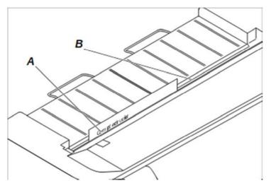
The paper is fed to the position where the bottom edge of the first printing line **A** is aligned with the tear edge **B** of the printer. The factory setting for the first printing position (TOF) is 12/72'' (4,23 mm/1/6 inch). This is equivalent to the second line from the top.
