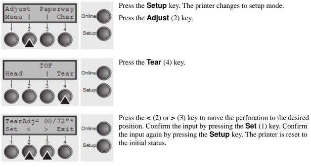
The correction made – a ma imum of appro  $\Box$  1" (2.5 cm) in each direction – will be retained after switching the printer off. It can be set separately for each paper path.
