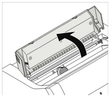
Before opening the cover, make sure that the printer is switched on so that it can e ecute automatic preparations for ribbon changing (widening the print head gap).
