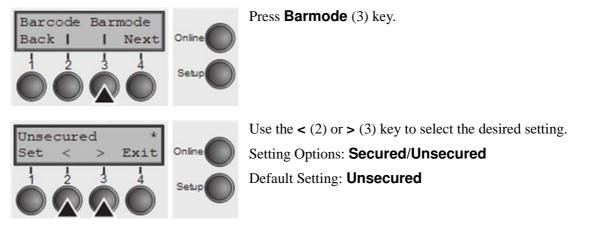
In **secured** mode, the space which the barcode characters require is "protected". In each line, other barcode or normal characters can also be printed. These additional characters are printed in the line currently being printed and and in the subsequent lines, without affecting the barcode which is already being printed. Consequently, normal characters can be printed in every line to the right or left of the barcode.
