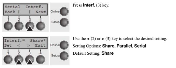
**Interf.=Share**: Printer switches automatically between parallel, ethernet and optional serial interface.
