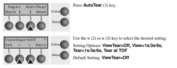
If the parameter **View Tear = Off** is set, the paper can still be brought into a View or Tear position via a specific sequence or the **Tear** key.
