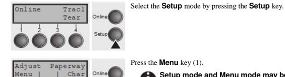
Setup mode and Menu mode may be disabled. Hold down the Setup key while switching on the printer to enable menu mode. If you want to enable access to this mode permanently, you need to change the appropriate setting in the menu.
