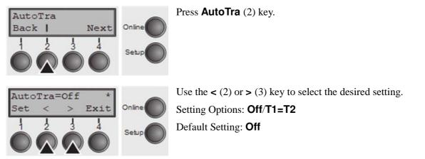
If an optional tractor is not installed, **Off** is displayed (factory default). If an optional tractor is installed and the **Off** parameter is activated, only the selected tractor is supported (either via the menu or an ESC sequence). If the selected tractor is out of paper, printing stops.
