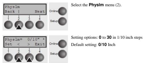
Permanent (physical) setting of the left margin. This parameter cannot be changed by emulation-dependent margin settings. Margin setting values entered by ESC sequences are added to the **PhysIm**.
