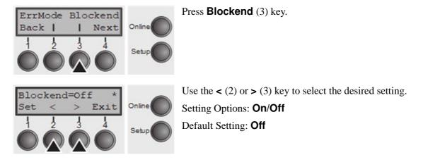
Confirm the setting by pressing the **Set** key (1). Press the **Next** key (4) to access the next group of parameters.
