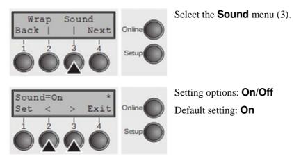
When **Sound = On**, a beep is generated every second to notify that paper is empty. Confirm the setting by pressing the **Set** (1) key. Change to the next parameter group with the **Next** key (4).
