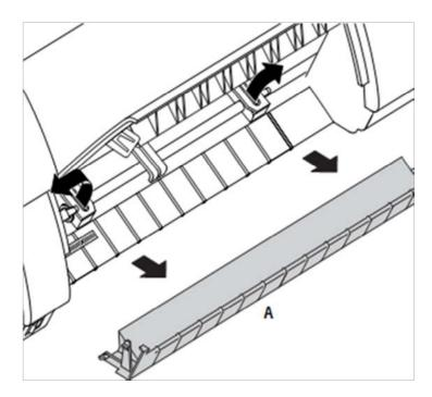
Open the front cover. Remove the bottom cover **A**. Open the right and left tractor flaps.
