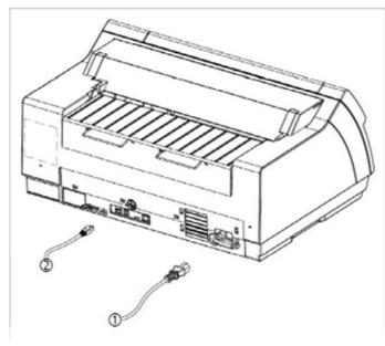
Connect the power cable (1) to the power inlet of the printer. Connect the power cable plug to a mains socket.
