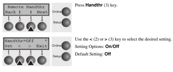
Confirm the setting by pressing the **Set** key (1). Press the **Next** key (4) to leave the parameter subgroup **Special**.
