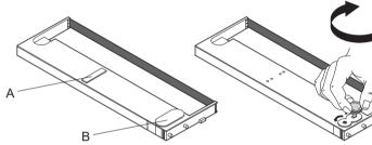
Remove green protections **A** and **B**. Insert green ribbon tension knob and tense ribbon by turning knob in the direction of the arrow.
