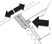
Open latch lever of righthand tractor. Align it to paper width. Insert fanfold paper into tractor. Make sure it is inserted by the same length as on left-hand tractor to avoid paper jam. Close flap and lock by turning lever to the rear.
