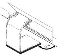
Make sure to align paper stack parallel with the printer and that paper flow is unobstructed. Lower front cover.
