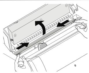
Switch on the printer. Open top cover. Move green friction tabs to the left and right and raise friction mechanism.
