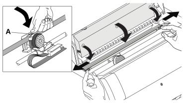
Press down green insertion tongue **A**. Move print head carriage back or forth and the ribbon motor will start to thread and tense the ribbon automatically. Press friction mechanism down until it clicks into place. Close top cover.
