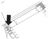
Open green latch lever. Align tractor so that first printing position on paper matches the **X** mark on printer housing. Lock lever. Place fanfold paper into lefthand tractor.
