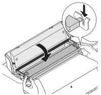
Slightly tilt ribbon cassette forwards and thread in ribbon between green insertion tongue and ribbon support (transparent plastic plate). Align and insert cassette into guides on the left and right. Press down until it clicks into place.
